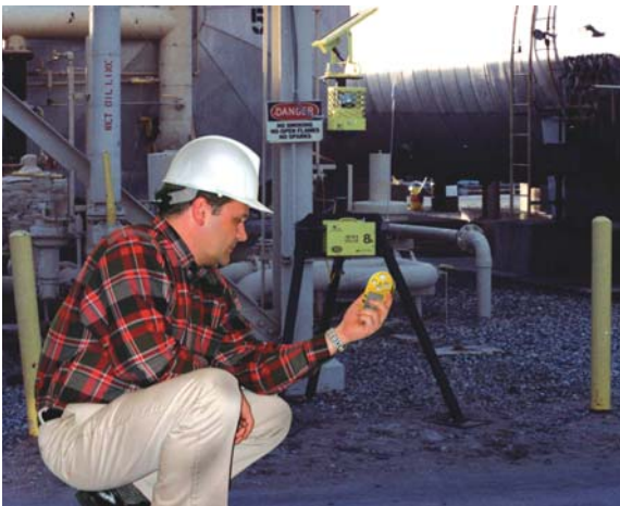
The best approach to VOC measurement is often a multi-sensor instrument equipped with both LEL and PID sensors
